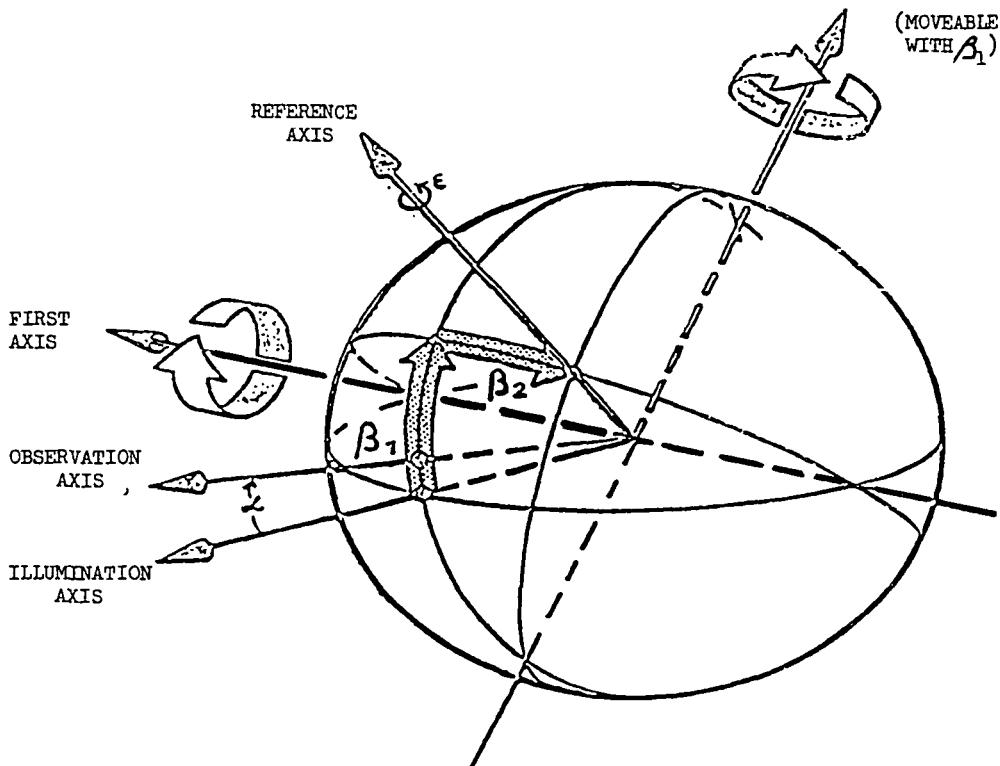
The CIE angular system for specifying and measuring retroreflectors. The first axis is perpendicular to the plane containing the observation axis and the illumination axis. The second axis is perpendicular both to the first axis and to the reference axis. All axes, angles, and directions of rotation are shown positive.
